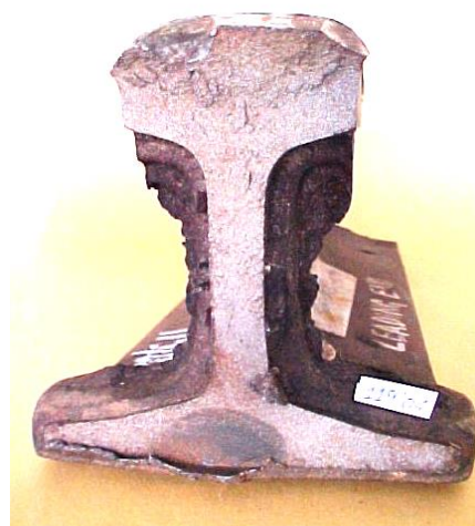
FIG. 51 : 421 - WELDING, THERMIT JOINT TRANSVERSE CRACK
