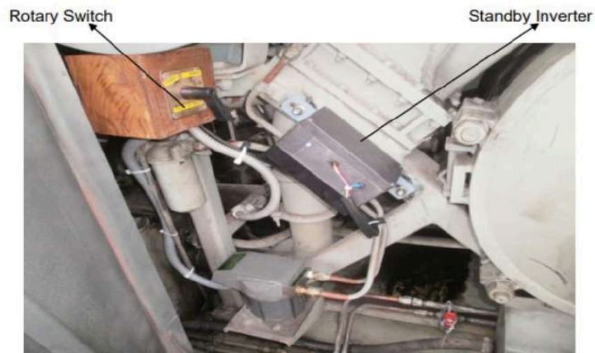
Fig.1 Location of fitment of inverter and selector switch
