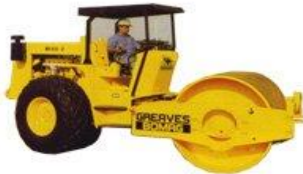
Fig-E9.3: Vibratory Rollers(Drum Type & used for better gradeability)
