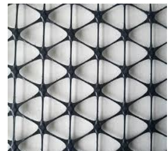
Fig-4.12 Geogrid with three axes
