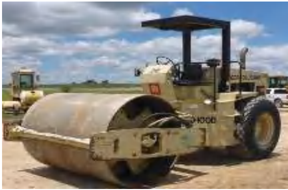
Fig-E9.1: (Drum Type & used for better gradeability)
