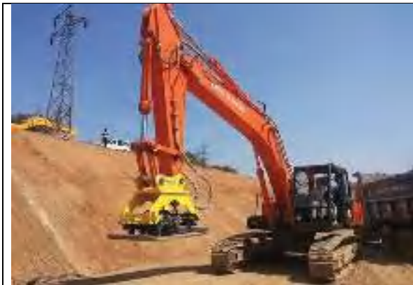
Fig-E4: Slope Vibratory Compactor
