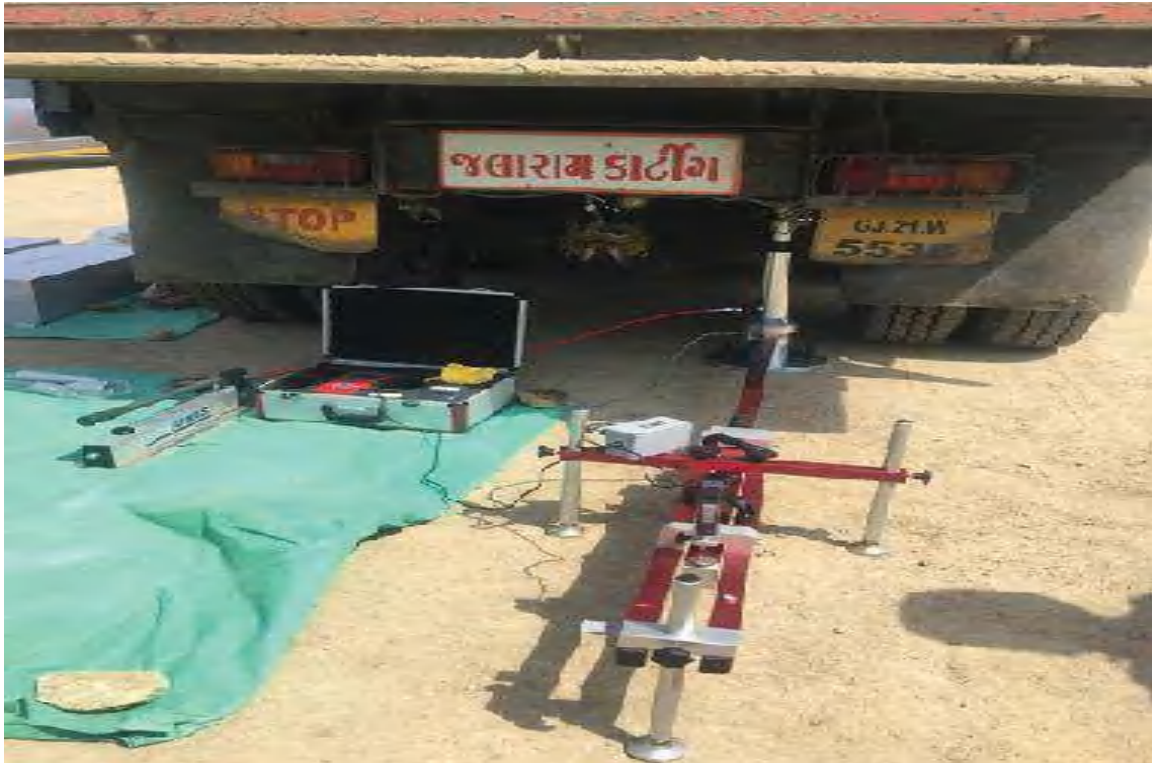
Fig-H 6: E_{v2} Measuring Equipment
