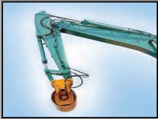
Fig-E2: Slope Vibratory Roller
