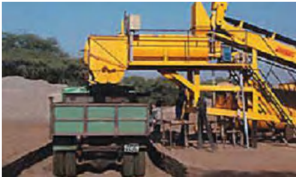
Fig-A6: Blanket Material Being Loaded into Truck
