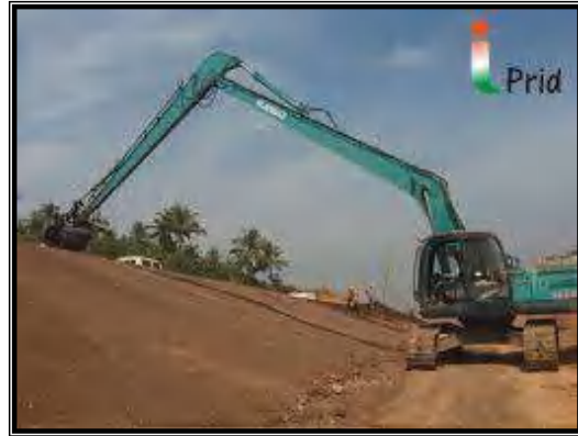
Fig-E3: Working of Slope Vibratory Roller
