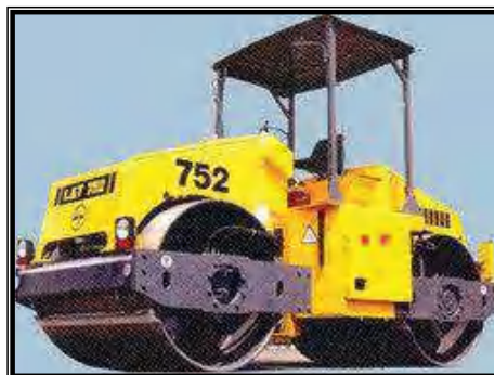
Fig-E8: Double Drum Vibratory Roller
