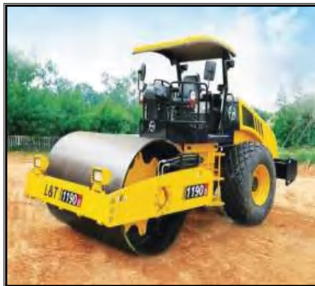
Fig-E9: Single Drum Vibratory Roller
