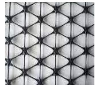
Fig-4.12 Geogrid with three axes
