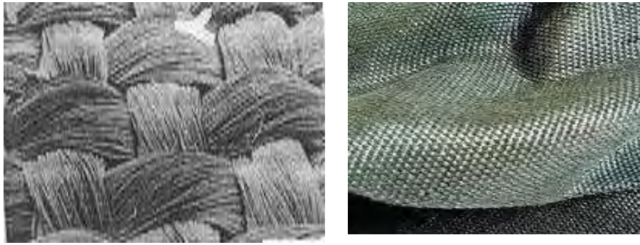
Fig-4.5 : Woven Geotextiles
