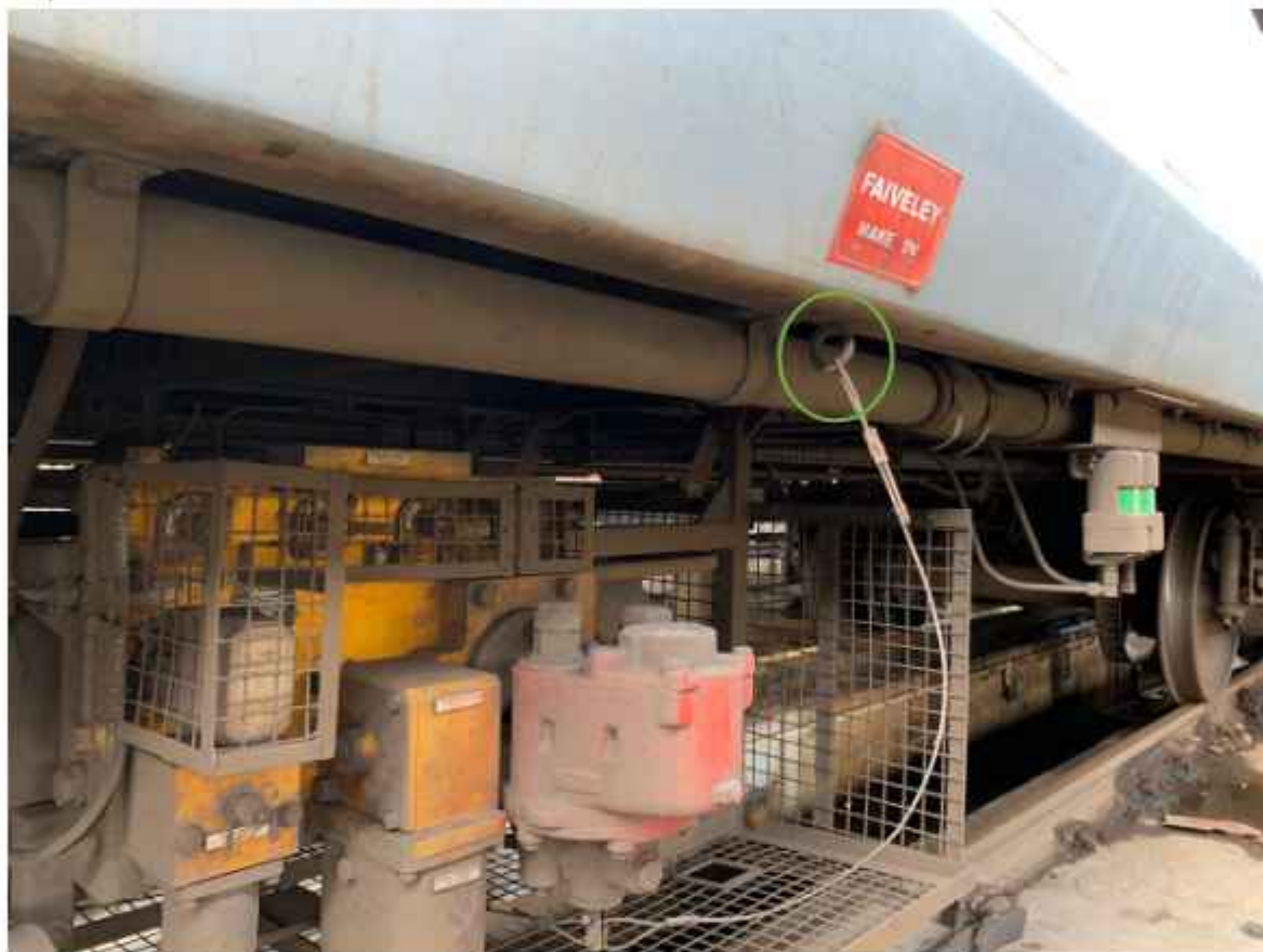
Wire rope arrangement (Brake Panel side)
