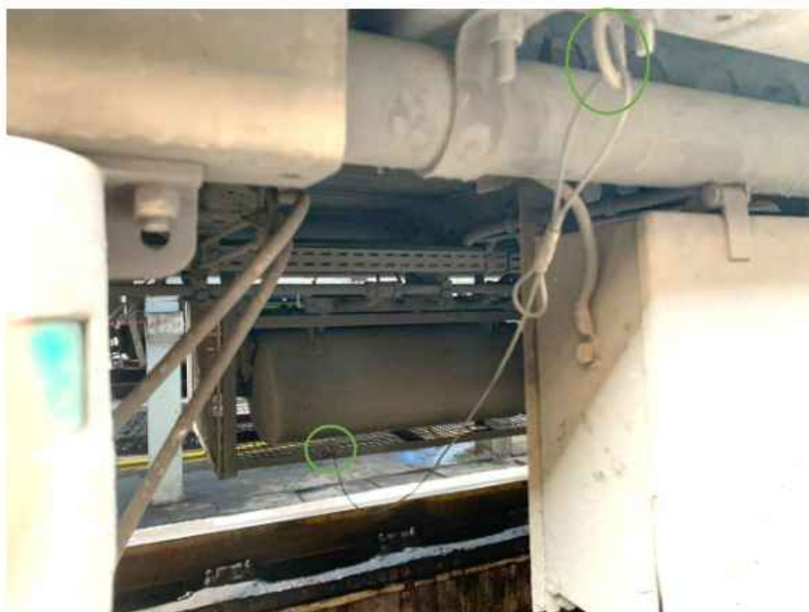
Wire rope arrangement (opposite side of brake panel)
