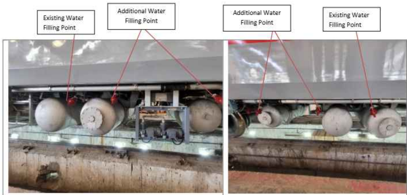
Fig-4 (Water Filling arrangements fitted on LHB ACCN Coach)
