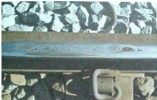
FIG. 40 : 2252 - HEAD SURFACE, WHEEL BURN REPEATED
