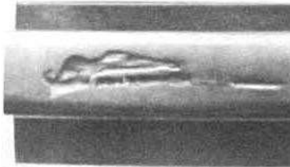
FIG. 36 : 1211 OR 2211 - HEAD, SURFACE, SHALLOW SURFACE DEFECT (FLAKING)
