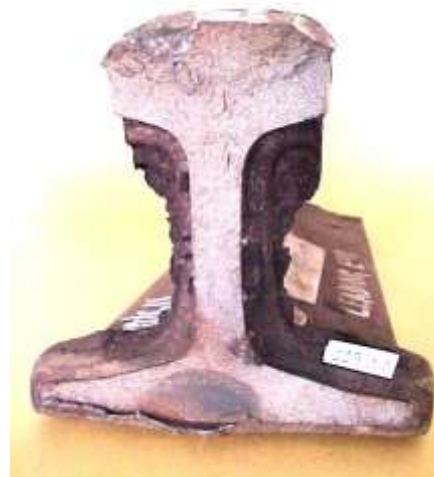
FIG. 51 : 421 - WELDING, THERMIT JOINT TRANSVERSE CRACK
