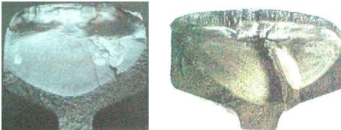
FIG. 54 : 471 - WELDING, BUILDING UP TRANSVERSE CRACKING OF HEAD ACROSS THE BUILT UP PORTION
