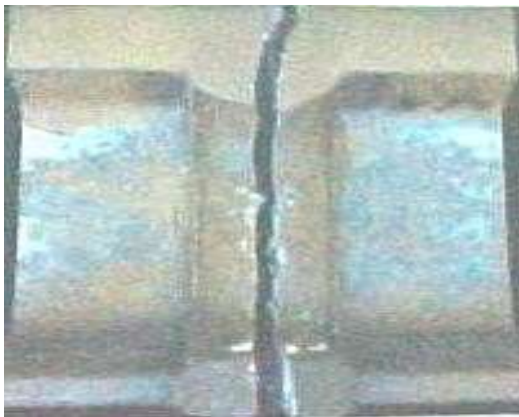
FIG. 50 : 411 - WELDING, FLASH BUTT JOINT, TRANSVERSE CRACK
