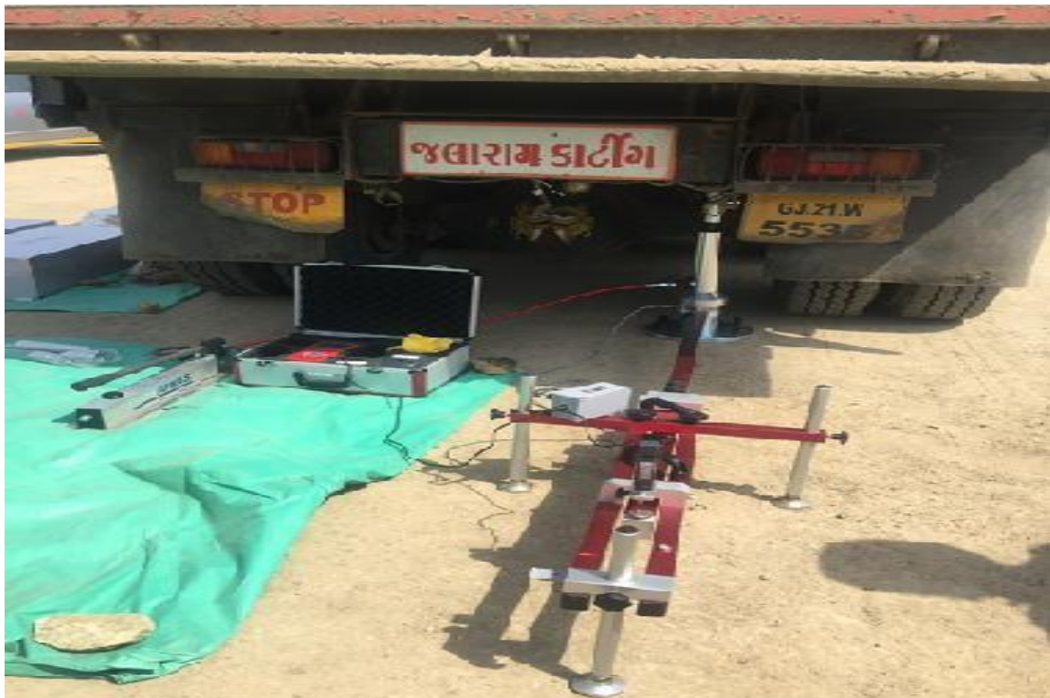
Fig-H 6: E_{v2} Measuring Equipment
