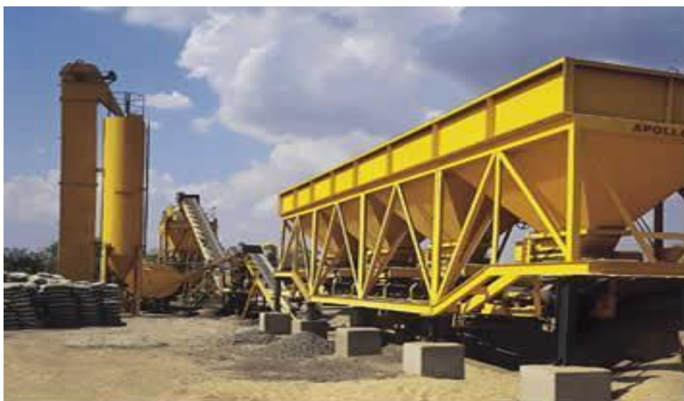
Fig-A5: Computer Controlled Bins for Mixing
