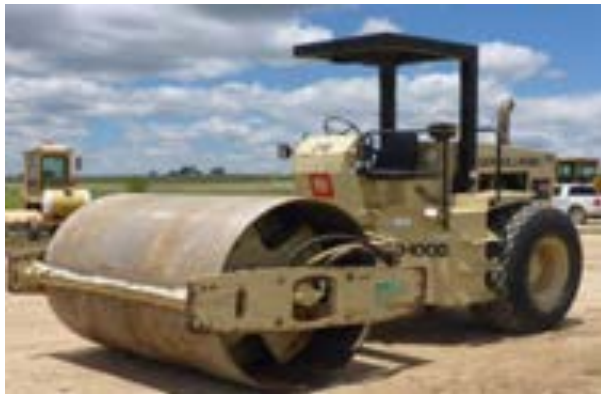
Fig-E9.1: (Drum Type & used for better gradeability)
