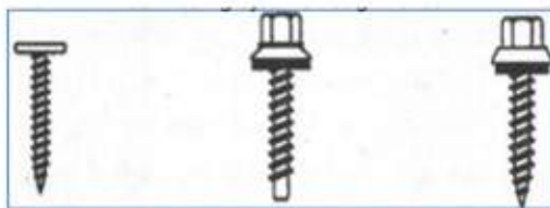
Fig 26.13A Self-tapping screw
