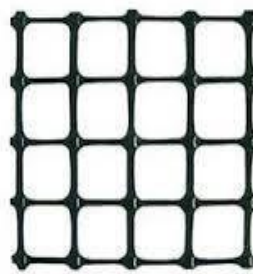
Fig-4.11 Geogrid with two axes
