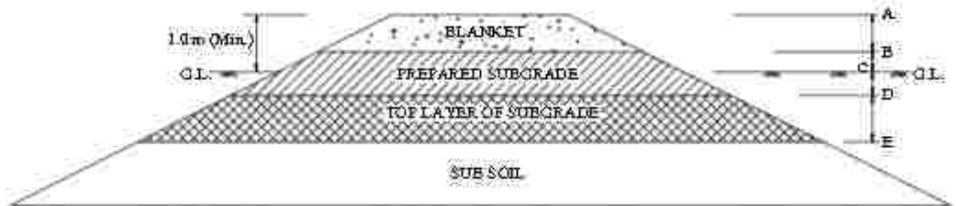
Fig-B 1: Formation Layers in Embankment
