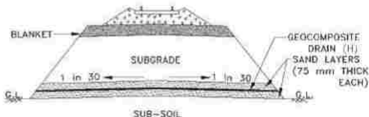
Fig-4.16: Use of Geosynthetic (Geocomposite drain-horizontal) in embankment over soft subsoil
