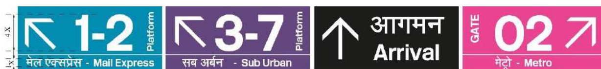
Figure 9: Colour scheme for zoning of different train type/traffic segment at complex station
