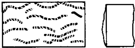
Fig. 7.2 : Hammer Dressed Stone Surface
