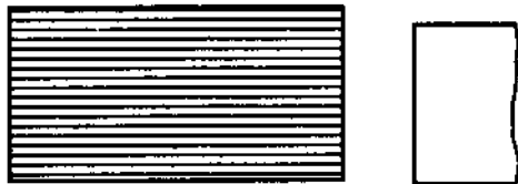
Fig. 7.6 : Closed Picked Stone Surface
