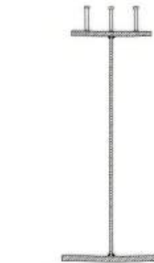
STUDS IF ANY TO BE WELDED AFTER COMPLETE FABRICATION OF GIRDER AT WORKSHOP OR SITE AS DESIRED
