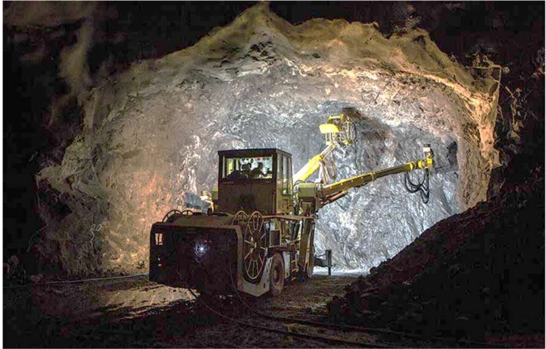
Figure 3: Face drilling using Boomer/Tamrock
