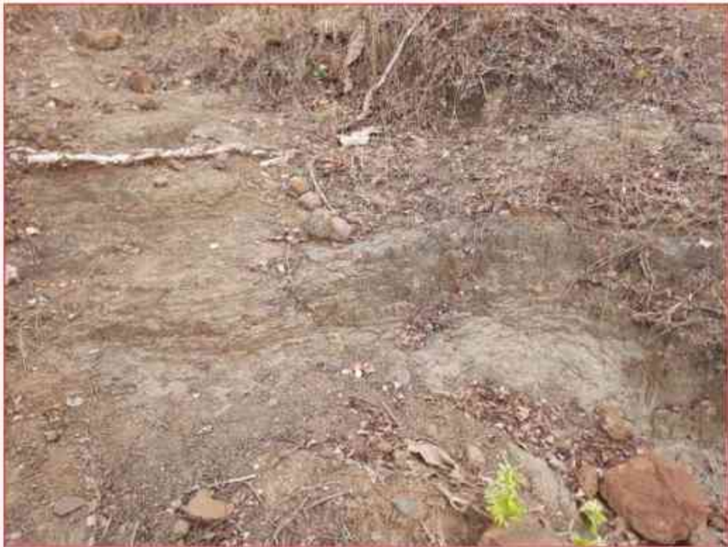
Figure 79 Scanty exposure of moderately to highly weathered Basalt.
