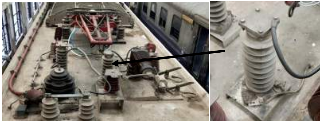
Figure 14: Lightning/ Surge Arrester
