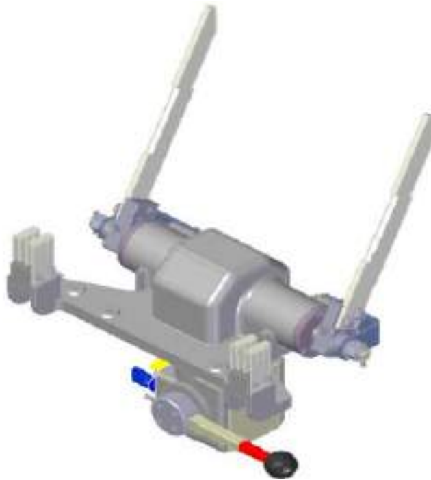
Figure 13: Earthing Switch for VCB
