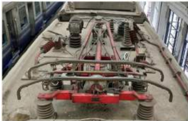
Figure 11: Pantograph at the Roof of Trailer Coach
