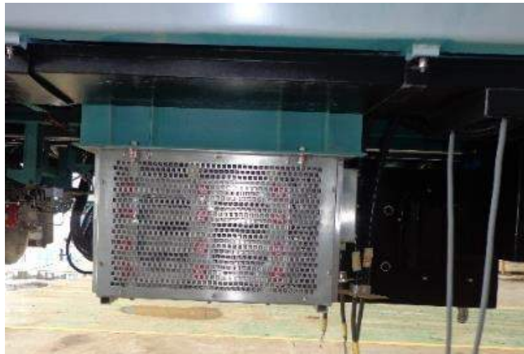
Figure 7: Brake Chopper Resistor
