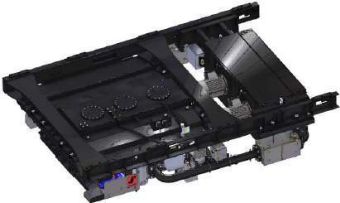
Figure 15 Traction Transformer
