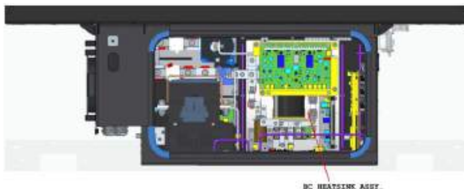
Figure 6: BC Heat Sink Assembly
