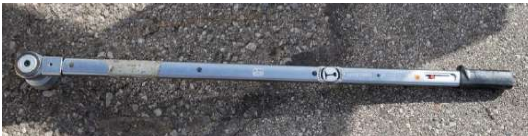
Torque Wrench capable for 580 Nm with Hexagonal 41 mm socket
