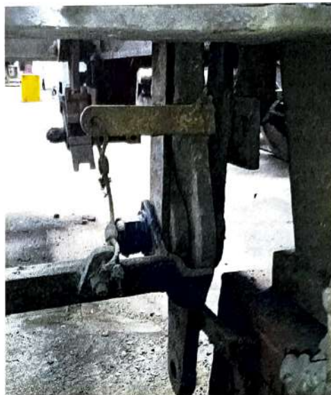
Fig.-2 Existing safety sling bracket location
