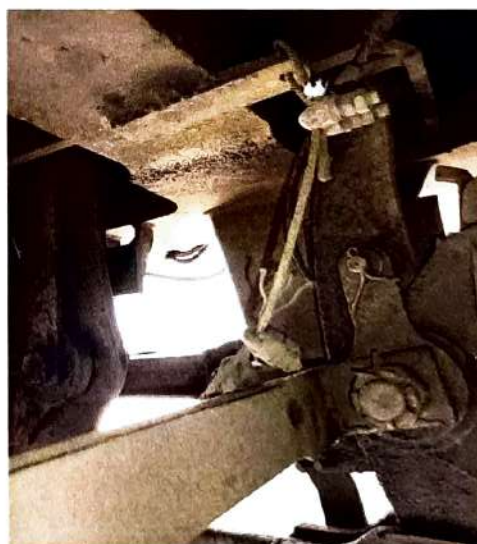
Fig.-4 Modified safety sling bracket location
