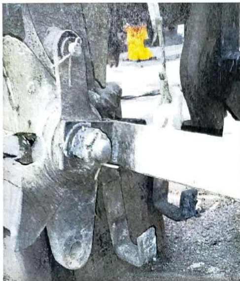
Fig.-1 Existing Tie-bar arrangement
