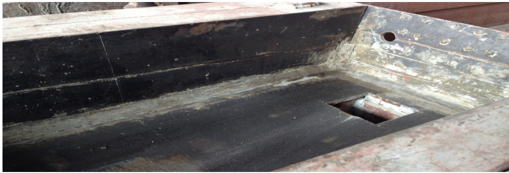
Offset kept in side plates in mould for producing concrete level guiding streak on the PCRSB ( for guidance only)
