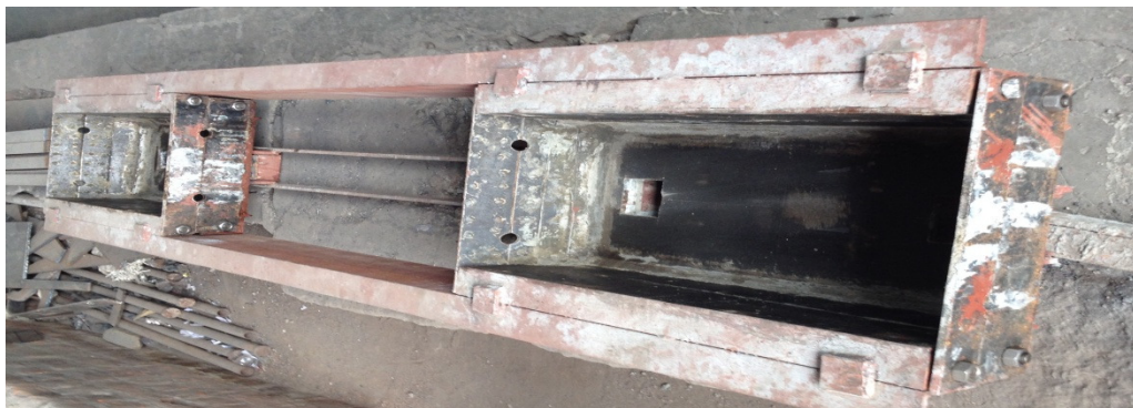
Sample mould for casting of PCRSB (for guidance only)
