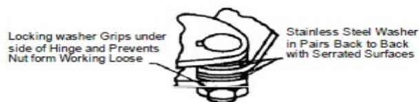
Fig. 21.14 : Illustration Showing Working Principle of Friction Stay
